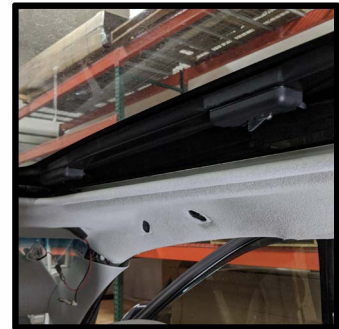
Sunroof trim and assist handles removed
